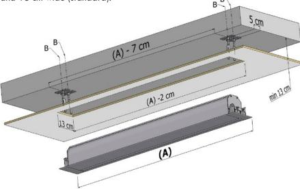
2. The fixing plates should be assembled as shown below.
