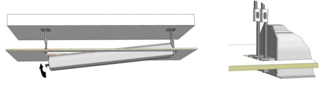
5. To make the screen flush with your ceiling, you need to turn the bolts to adjust the height of the screen casing. MAKE SURE THE SCREEN IS LEVEL!
