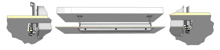
6. Put the parts of the cover plate in place to hide the fixation brackets.
